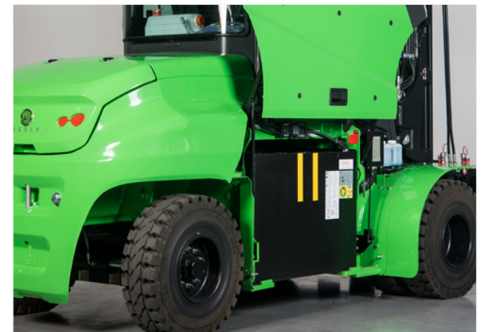
Open chassis design with side panel facilitates lateral battery exchange.
